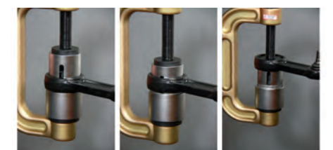
bush extraction on suspension arm
