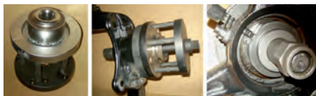
assembly preparation bearing-ø 72 mm, disassembly bearing-ø 85 mm (hub view), disassembly bearing-ø 85 mm (rear view)
