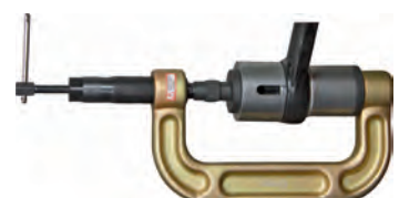
applying hydraulic spindle 5501 with press and pull sleeve set 5505
