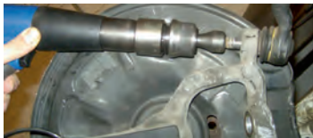
track rod end removal (with No. 8760)
