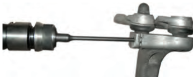
clamp bolt removal (with No. 8751)
